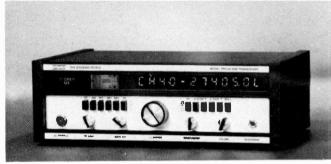
quency on both receive and transmit. The channel numbers are also indicated, as well as the sideband in use. The display is driven by the microprocessor, which autotracks when the channels are changed.
