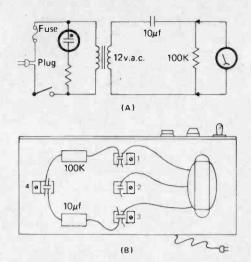
Fig. 2(A)—Circuit used to observe the effect of the reactance of a capacitor. (B) Pictorial set up of the circuit of (A).
