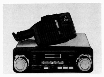
to-talk" control, RF gain, and a bright LED channel readout, making the 615CB convenient to use even while driving.
