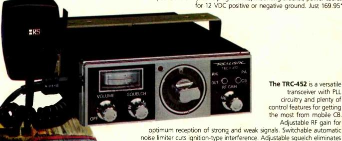
The TRC-452 is a versatile transceiver with PLL circuitry and plenty of control features for getting the most from mobile CB. Adjustable RF gain for
