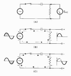
Fig.4.49(A)—Circuit used to couple AC to a load through a capacitor. (B) First half of the AC cycle charges the capacitor causing a current flow through the resistance. (C) The second half of the cycle causes the capacitor to charge to the opposite polarity and reverses the direction of the current flow in the circuit.
