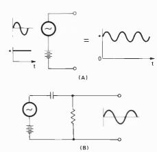
Fig. 4.50(A)—Placing an AC voltage and a DC voltage in series results in a pulsating DC voltage. (B) Coupling a pulsating DC through a capacitor permits only the AC to pass and appear as output across the resistance.
