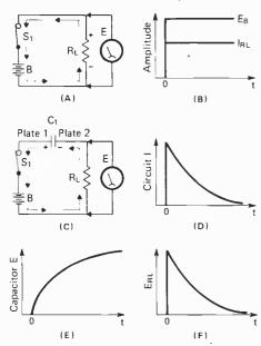
Fig. 4.48(A)—DC voltage is coupled directly to load through the switch and wires. (B) Plot of E and I VS. time. (C) Insertion of capacitor blocks DC from load. (D) Plot of circuit current shows no flow after capacitor charges. (E) Plot of capacitor charge VS. time. (E) Plot of output voltage versus time shows no voltage after capacitor charges.
