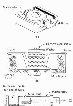
Fig. 4.43(A)—Appearance of a typical compression trimmer capacitor. (B) Construction of a compression trimmer capacitor. (C) Construction of a piston trimmer capacitor.
