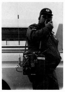
"The Box" has a unique lid that doubles as a pocket for excess antenna wire or carrying misc. items. Radios are mounted in "The Box" by special shock foam, giving the S.B. 360° ventilation and protecting it from road vibrations, hard knocks, etc. Installation requires a sharp knife and takes approximately 5 min. Accesories for "The Box" are a 12 Volt battery pack and antenna (magnetic) mount.
