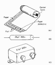
Fig. 4.35(A)—Method of forming a paper capacitor. (B) After the capacitor is rolled and leads attached it is dipped in a wax or plastic to insulate it. (C) A "bathtub" type capacitor.
