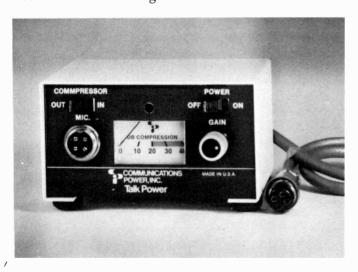
By way of contrast, the CPI speech processor follows a *logarithmic* curve allowing high gain on the lower and intermediate audio levels (which contain much of the human speech information) but smoothly leveling off—compressing gain as the level increases (See Figure 6). Overshoot on the peaks is impossible. Incidentally, correct attack and delay times are essential and these are carefully controlled factors in the
