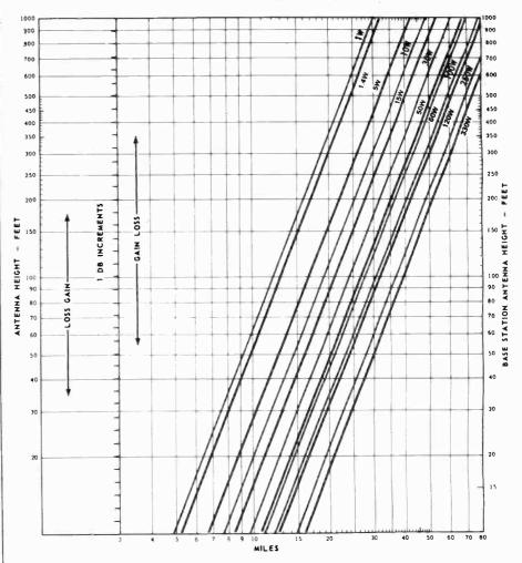
Chart based on propagation calculation procedures developed by Kenneth Bullington, Bell Telephone Laboratories, with correction factors added to compensate for losses experienced in average actual situations.
