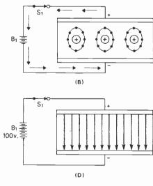
Fig. 4.26(A)—Basic circuit for charging a capacitor described in the text. (B) With S<sub>1</sub> closed capacitor charges, as described in the text, and causes eliptical orbits of the valence electrons in the dielectric. (C) Electric field exists between the two capacitor plates. (D) Increasing the applied voltage increases the strength of the electric field. (E) When S<sub>1</sub> is apened the charge remains an the capacitor; energy is stared in the electric field.
