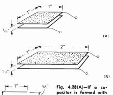
(C) Another method to increase plate area that only increases the thickness of the capacitor.
