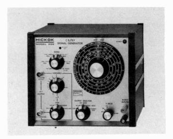
receiver sensitivity checks. The attenuated output is variable in 20 dB steps and by a 20 dB continuously-variable control calibrated in microvolts.
