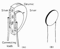
Fig. 4.37(A)—Cross section view of a disc ceramic capacitor. (B) Dipped and sealed ceramic capacitor.
