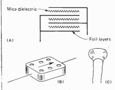
Fig. 4.36(A)—Construction of a mica capacitor.
