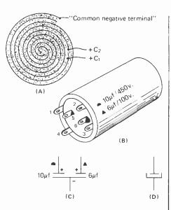
Fig. 4.40(A)—Cross section view of a dual capacitor dry electrolytic. (B) Typical aluminum can housing for the dual electrolytic capacitor. (C) Circuit symbol for the dual electrolytic capacitor housed in the can. (D) Symbol used to specifically indicate an electrolytic capacitor. The short line is the positive terminal.
