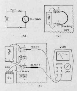
Fig. 1(A)—Circuit to test capacitor charging action. (B) Pictorial of test set up. (C) Jumper used to short circuit the capacitor.
