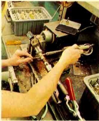
Archer antennas are hand-crafted for quality. This expert is putting the final touches on loading coils.
