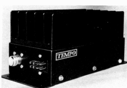
Fig. 2—Solid-state linear amplifiers such as this will step up a 5 watt mobile signal to 100 watts at 2-meters.
