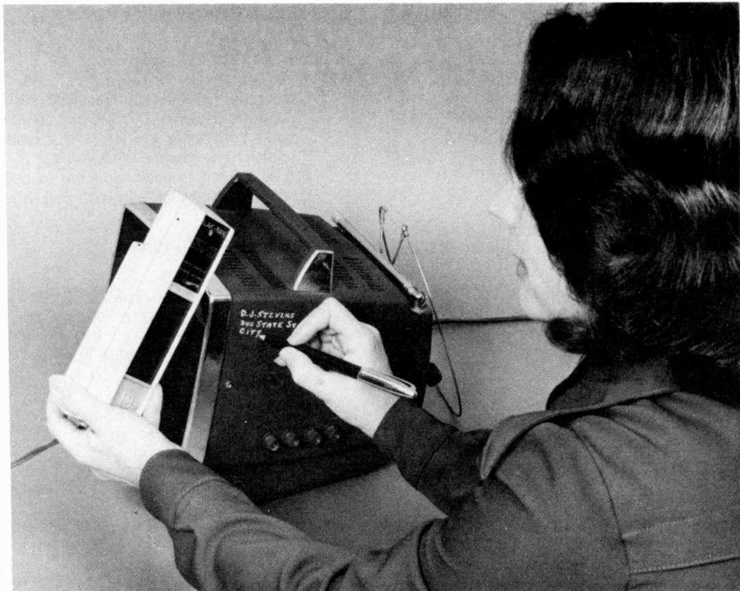
One novel method of marking up equipment for later recognition is by marking it with invisible ink which will show up under special light.
