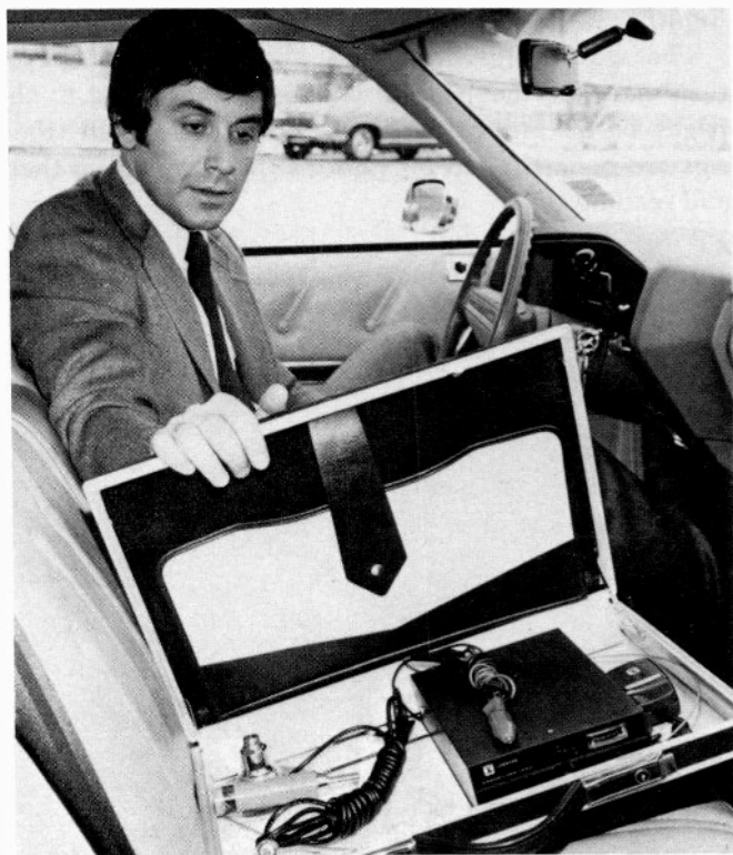
A totally portable CB station, as removed from a vehicle for security purposes. The antenna has a magnetic base and breaks-down, the rig slips out of the mount and into an attache case for assurance that when you get back to your car you'll still be a CB'er.
