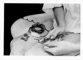
TERI could have chopped the wire ends cleaner with diagonal cutters. The important thing, however, was to have the wires equal in length.
