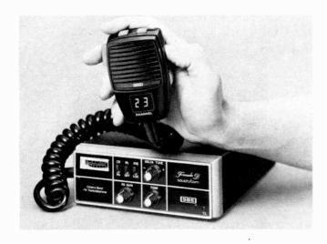
daylight viewing. Full range volume and squelch thumbwheel controls, both fully adjustable, are located on the right side of the microphone. A push-to-talk switch is located on the left.
