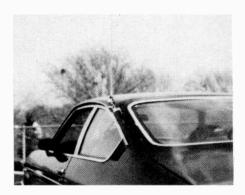
The "static ball" tuning tip eliminates the need for cut-and-try antenna trimming. Once the desired setting is achieved, the static ball can be secured in position with an allen wrench that comes with the antenna.
