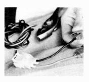
Splicing two wires together this way entails laying one wire in the goove; snapping the little side gate shut on it; then poking the other wire into the end hole and squeezing the cover flap till it clicks. Metal
