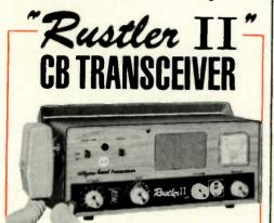
11115 5 WATTS -**11 CHANNEL POSITIONS TUNES ALL CHANNELS – "S"/RF METER**
