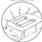
The DDRR Antenna been designed to incorporate the electromagnetic efficiency of naturally resonant quarterwave whip antenas with a low profile which can be easily installed on vehicle roof tops and precisely tuned over a wide range of frequencies. Because of its unique design features, the DDRR Antenna will normally outperform quarter-wave mobile installations, both in transmit & receive modes. Other frequencies available —from 27 to 180 MC. CB Net \$29.95.
