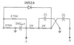
For those living in noisy locations, the following noise circuit is worth while. The entire circuit is built on a terminal strip and mounted on the chassis and then inserted into the circuit as shown in figure 3.
