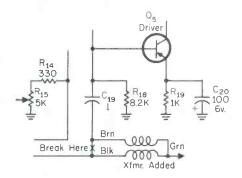
secondary impedance of 8 ohms. The centertap is not used. Of course there is a slight mismatch but only approximately 2 to 1. An increase of 30% to 40% modulation was observed on the oscilloscope. This transformer was also used because of its subminiature size. It can be mounted almost anywhere in your walkie-talkie.
