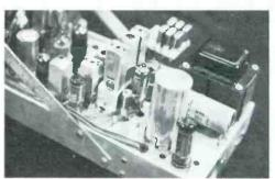
One sure-fire way to judge the relative sensitivity and selectivity of two receivers is to compare the number of IF (intermediate frequency) stages of each. Thus the Johnson Messenger I CB transceiver has one IF stage while its more expensive successor, the Messenger II has two such stages. The extra tube and four tuned circuits (two in each IF can) give much improved sensitivity as well as selectivity—freedom from adjacent channel interference.
