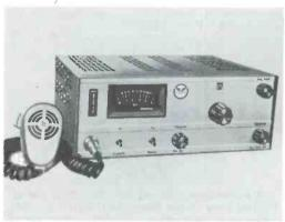
Browning Laboratories, Inc., Dept. S9, 1269 Union Avenue, Laconia, N. H. has released some details on their exciting new *Raven* transceiver, a self-contained mobile unit. Special features include an "opto-electronic automatic compressor;" a two Nuvistor cascode front end; twelve tubes with 19 functions, two transistors and five diodes. There are no synthesized circuits.
