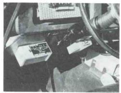
Photo of a complete convertized mobile unit. On the left is a Hartman marine converter, in the center a Sentry Electronics police model, and on the right an International Crystal unit for aeronautical frequencies. These units are top-notch and can be recommended highly from personal experiences with them. A Crescent Electronics unit is in use at the base station.
