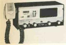
Allied Radio, 600 North Western Avenue, Chicago, Ill. 60680, has come up with the Knight KN-2590 Dual Power 8-channel CB rig which features a switch for a choice of 100 milliwatt or 5 watt input. The receiver is tunable across the entire 23 channels. The transmitter includes speech clipping for maximum effectiveness at 100% modulation. Price is \$79.95, factory assembled.
