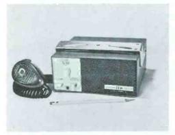
The Squires-Sanders 23'er. Note its small size compared with the pencil in the foreground. For base station use is locked on top of a 2-inch-high tilt-up base (not shown) which contains a 117 v.a.c. power supply.
