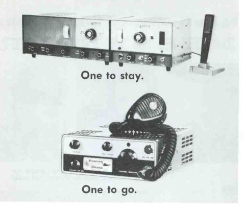
The Browning Eagle CB base station is perfectly happy to stay at home or place of business. The receiver has RF gain control, selectivity switch for broad or narrow selectivity, cascode nuvistor front end, 12 tuned I.F. coils. The transmitter has clipperfilter stage, built-in SWR meter and 23channel operation. Everything's complete, no extras to buy. Best performing base station you can get ... at any price. It's bound to be better, it's by Browning!
