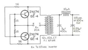
Number 2 on my list of possible solutions is to build up a 6-volt to 117-VAC inverter, using the circuit shown in the other schematic. This one would cost you quite a bit more, though. The transformer alone would eat up your budget, and the transistors cost from \$3 to \$5 each, depending on how lucky you are. I really think you'll find the double-battery route the best.
