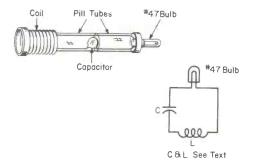
posite sides which are made with a heated pin) solder a 10 uufd mica or ceramic capacitor.
