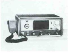
The KN2565 is among the latest additions to the third generation of CB transceivers, and typical of these units it is supplied with complete 23 channel coverage via frequency synthesis.
