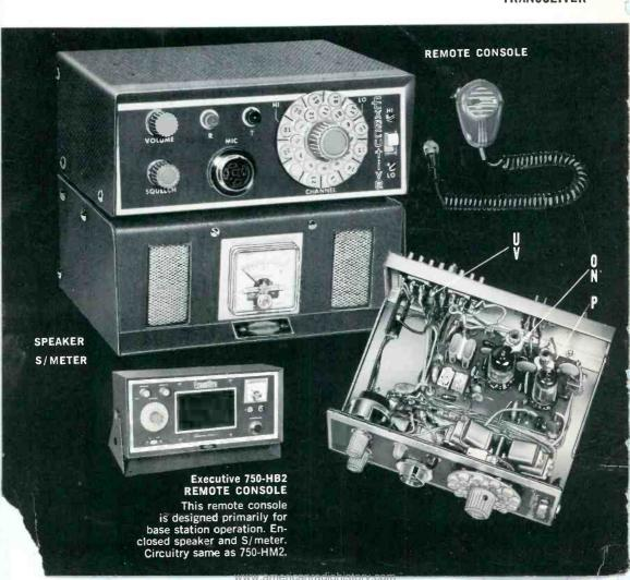
a\sensitive and selective dual conversion receiver combined with a highly stable and efficient transmitter. The 23-channel crystal controlled transmit and receive frequency selector circuits are housed in the remote console. • Features include a new delayed / expanded AVC, new speech clipper/filter amplifier, new built-
