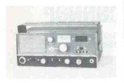
The USL Contact-8 CB Transceiver. At the bottom from left to right are: mic connector, CB-PA switch, volume control with power switch, spotting switch, receivertunina or crystal-control switch, channel-crystal selector, headphone jack. The squelch control is at the right of the speaker grille with the tuning dial just at the right of center. Below the meter is the meter function switch along with the two external-crystal sockets below it.
