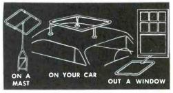
noise pickup. Not so with the horizontal antenna. Lying flat, it creates cross-polarization; noise is vertical, antenna horizontal. Electrical hash is knocked down many db.
