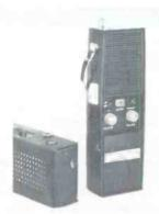
Raytheon Company, 213 E. Grand Ave., South San Francisco, Calif. has a new 2 watt hand held transceiver using 13 transistors, 2 diodes and a thermistor. Called the RAY-TEL TWR-6, the set weighs in at 2¾ lbs. A meter on the side of the set shows the amount of charge of the self contained nickel-cadmium batteries. The batteries are recharged from any household wall outlet. Suggested price is \$119.50, plus optional accessories. Contact Dave Thompson for more details of this miniature powerhouse.
