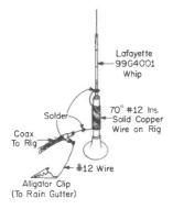
The loading coil consists of 70 inches of No. 12 insulated antenna wire, wrapped tightly around the dowel, with about 2 inches left at each end.
