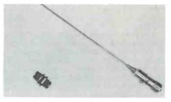
The Toroid-Tenna. It is trimly styled with the toroid transformer enclosed in the base with a tuning adjustment accessible through a small aperture at the projection on the side. The base is fitted with a PL-259 coax connector. A suggested mounting accessory, an 83-IF coax adapter, is shown at the left (not supplied with the antenna).
