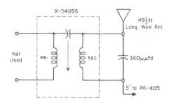
coil in parallel hookup we used a 360 uufd mica capacitor (Lafayette 30-G-3541, 53¢). The wire for the rest of the antenna: anything you have kicking around the shack which is of sufficient
