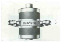
ful AM broadcast stations) and millions of watts of pulse power. Widely used in long-range radars, space research, and nuclear particle accelerators. Although the 3.5-volt filament voltage of the 7835 appears modest, the filament-current rating is a whopping 6600 amperes—more than 2300 watts for the filament alone. Price: \$7800-\$64000.
