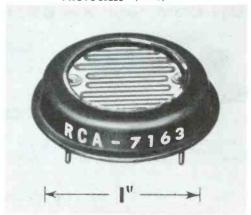
Members of this family may be found in use almost everywhere. Applications include auto headlight dimmers, doon openers, streetlight controls, bowling foul-line indicators, and sound-on-film detectors. Fundamental principle is that of a resistor whose resistance varies with the amount of light falling on the light-
