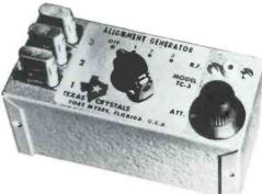
The model TC-3 oscillator has been announced by Texas Crystals, 2100 Crystal Drive, Ft. Myers, Fla. This is an ideal unit for aligning an IF strip, for use as a signal generator, as a marker generator or signal source—in fact, it can be put to numerous uses on any frequency between 200 kc/s and 3 mc/s. Price is \$29.95 (including batteries and 3 standard frequency crystals).
