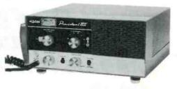
Here's a new rig from GC Electronics, 400 S. Wyman Street, Rockford, Ill. The set is known as the "President VIII," and features 8 crystal positions, an external crystal socket, a tunable receiver (with crystal spotting, an S-meter, PTT, universal power supply, adjustable squelch, 18 tube performance. Further details and price were not announced at press time but are available from the company now.
