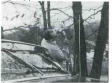
The field-strength meter, as most CBers already know, is a gem for checking direct radiation from a mobile whip. Yet the gadget easily gives all sorts of misleading indications when not handled properly. Here are some items to watch out for. They can help make the instrument far more valuable than any number of S-meter reports on transmitter tuning, whip length or other factors affecting mobile antenna performance.
