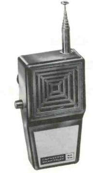
for a pair, the unit is compact in size, utilizes 3 transistors, push-to-talk, and weighs a mere 1 lb. Operates from a single 9 volt battery
