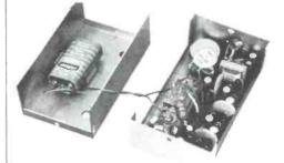
Interior view of the Model C-II. The three transistor stages are mounted on a small printed-circuit board at the right. The other round ended objects are tiny electrolytic capacitors. A 9-volt transistor-radio battery is held in the cover at the left.
