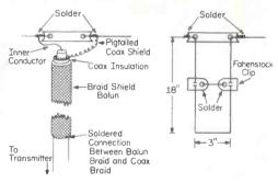
Transmission line with balun (before weatherproof wrapping). On the right is the tuning stub with sliding short.
