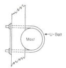
Top view of 2 x 2 wooden boom grooved and bolted to mast.
