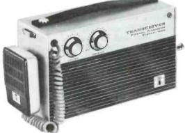
This month we put the Inter-Mark Cipher 1000 through its paces in the S9 Lab. The rig is a portable Class D unit which is operated from 18 volts worth of flashlight batteries or from an external AC power supply (optional accessory).
