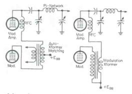
deliver the necessary peak voltage for strong modulation, it must also work into a specific value of load resistance. These two resistance values are usually not of the same value. As a result some form of output modulation transformer or auto transformer must be used. The two basic circuits common to CB equipment are shown in Fig. 2. Proper operation of the modulation system thus depends on correct impedance matching and an adequate modulating signal level.
