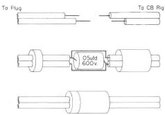
of those cylindrical plastic pill bottles which most drug stores keep in stock. A hole is drilled in the bottom of the bottle and also in the cap and these are placed on the power lead before the capacitor is connected. The bottle must be at least I" long by ½" in diameter to enclose the capacitor.
