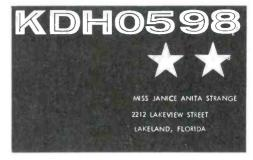
A line negative used for the contact printing of postcard QSL's on sensitized stock.
