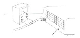
jacks. Actually the wire should be twisted into a loop of several turns and placed near the rear of the transceiver or wrapped loosely around the coaxial cable.
