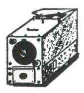
The going price for a used, but excellent condition, BC-455 is about \$10, plus a power supply to operate the receiver from 117 volts AC. It will have to furnish 6.3, 12.6 or 24 volts for the filaments and 250 volts for the plates (these are also available on the surplus market. The only other parts you will need are a phone jack, plate switch, midget 25,000 ohm pot, a 5 prong socket with male plug to match power connections at the rear of the chassis and a splined turning knob.
