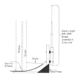
A mounting brace was made out of 1" pine wood, as shown in the illustration. This brace is held in place by the window being closed down on the "U" shaped section. The antenna is fed with RG-58/U, with the shield (in my particular instance) being connected to the window screen in back of the whip. I suppose that a connection to a radiator or water pipe would give better results, however none happen to be convenient to the window I am using. As short a lead as possible to "ground" is suggested.
