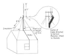
Instead of an actual whip, you might try using a length of ½-inch aluminum electrician's conduit, or, for a little more money, the same size tubing made of the stiffer alloys of aluminum.
