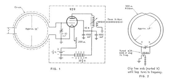
CB'ers have requested information and construction information on direction finding loops to use in locating mobile units, determining the direction of base stations, for tracking down sources of interference.
