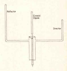
Fig. 5. Vertical Beam Antenna With Coaxial Dipole
