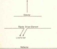
Fig. 1 The Three Element Beam Antenna
