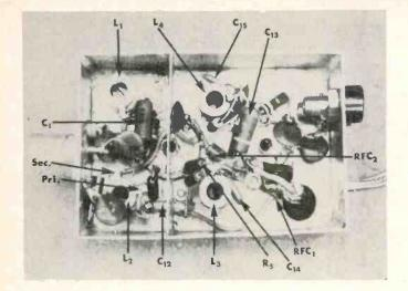
Fig. 5. Bottom view of wired chassis. Main components and their locations are identified.
