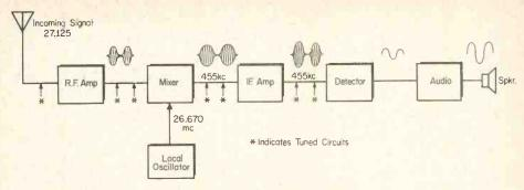
Fig. 1. Block diagram of a typical CB receiver.
