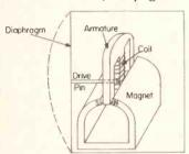
Fig.6- Controlled Magnetic
