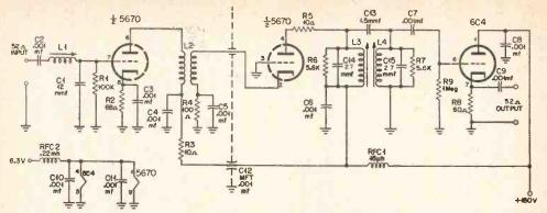
Fig. 1. Final circuit using cathode follower output. Although not shown, pin 5 of the 5670 should be soldered to the shield.
