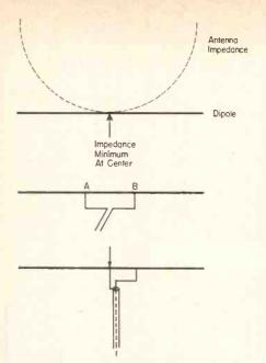
Fig. 3. The Gamma Match For A Beam Antenna
