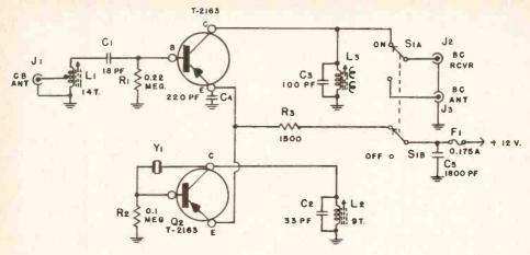
Fig. 2. Schematic diagram of 9W0831's "mini-verter."
