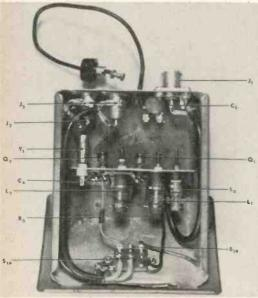
Fig. 1. Here's the "mini-verter" built into a car's ashtray.
