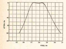
Fig. 2. Overall response of preamp.
