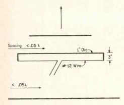
Fig. 4. Closed-Spaced Beam
