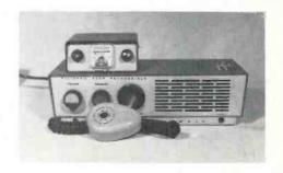
is a combination preamplifier-compressor with a *calibrated* percent modulation meter (*Communications*, *Inc.*, 33 Danbury Rd., Wilton Conn.).
