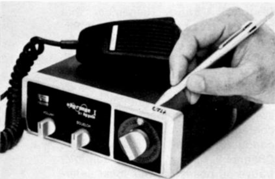
Mark your CB unit with an engraving tool.
