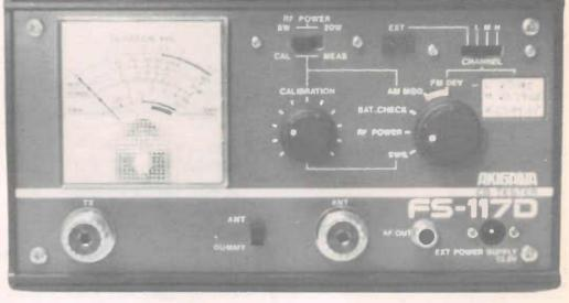
he Akigawa FS117D is one of those small boxes designed to combine several measuring facilities in one unit. The introduction in the instructions says it is "the all-round tester for 27MHz band AM/FM transceivers." On offer here are provisions for measuring RF power up to 20 watts, standing wave ratio, AM modulation depth and FM deviation on selected channels. All measurements can be taken into the internal dummy load if required.
