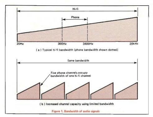
Channel 2 goes through a converter that shifts everything up by 5kHz, so that this channel now occupies 5kHz to 10kHz. Similarly channel 3 is shifted up by 10kHz to occupy 10 to 15kHz and channel 4 is shifted by 15kHz to occupy 15 to 20kHz.
