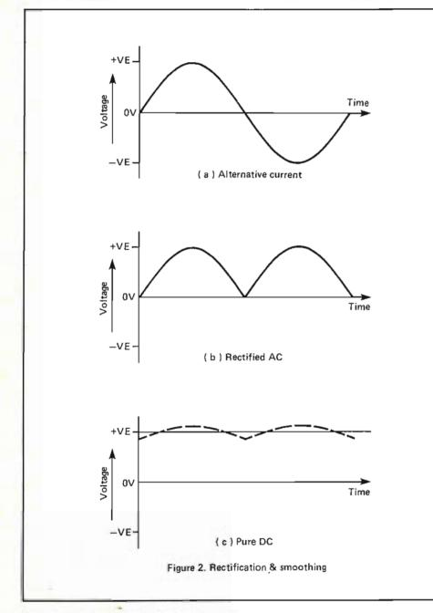
emerging. When the top end of the winding is positive and the bottom negative as shown the current flows through D2 and D3 which are forwardbiased. D1 and D4 are reverse-biased in this condition. During the next halfcycle when the positive and negative from the transformer are reversed, the current flows through D1 and D4, and D2 and D3 are cut-off. The output with this circuit is identical to that for the rectifier shown in Figs. 1 & 3.
