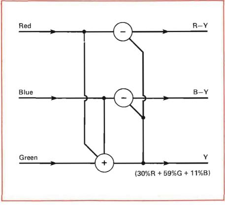
Figure 7. Obtaining colour-difference signals
