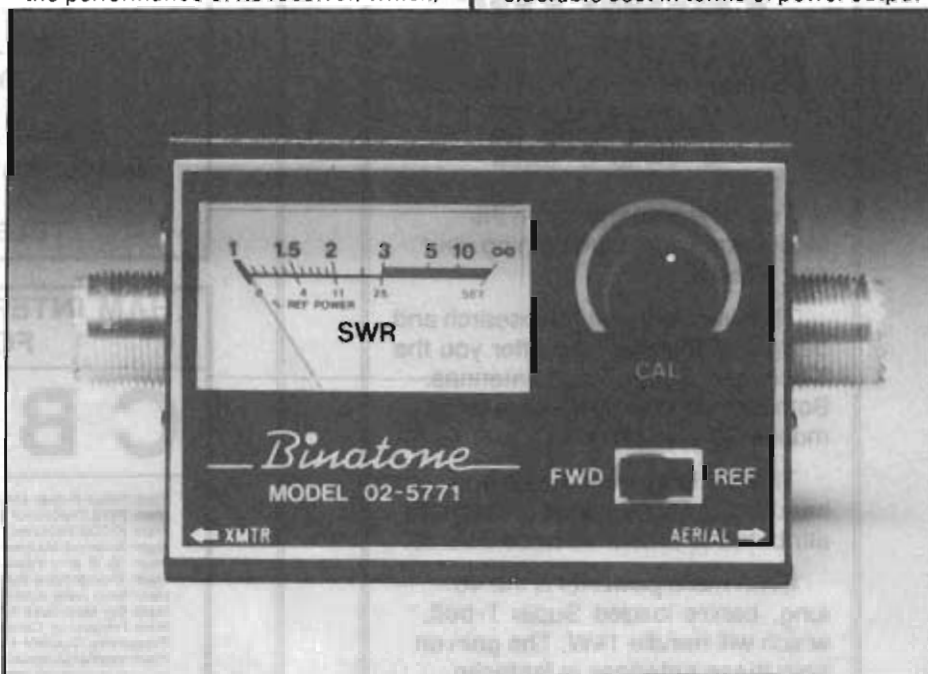
Leaving an SWR meter permanently in-line means reduced transmitted power
