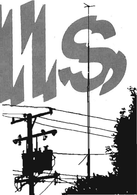
Keep antennae well away from power lines. If the mast touches the cables sparks will fly.
