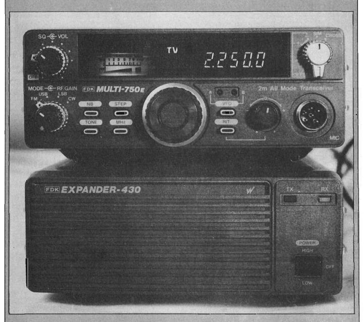
Another mobile or base station with a UHF adaptor. The transceiver features 10 watts on FM/ SSB/ CW 144-146MHz. The adaptor gives operation in the UHF band 430-440MHz by a press of a button.
