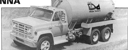
So where would you put the antenna on this vehicle? Remember various ground plane heights can cause SWR adjustment problems as well as giving an unsymmetrical radiation pattern.
