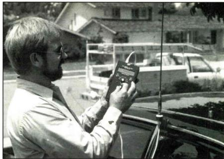
The MFJ SWR Analyzer is a fast way to check a mobile CB antenna's resonance.
