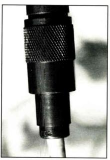
Rainwater got into this open coax connector and SWR went off the scale!
