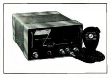
This 30 watt five-channel 27 MHz AM transceiver was made by CB manufacturer e.c.i., supposedly for commercial two-way users. CBers bought all of them.
