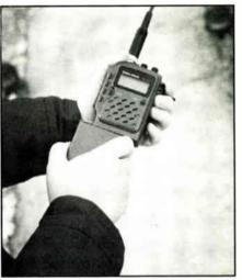
Unlike the RadioShack amateur HTs, the battery pack on the TRC-232 slides off from right to left. It's a bit awkward, requiring a good grip on the radio portion of the unit
