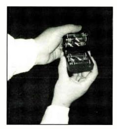
Here's a look at the 6 "AA" alkalines in the battery pack. Always use alkalines or (in the other supplied battery case) NiCds, and NEVER mix types of batteries! We found the battery cases somewhat difficult to open; for this reason we suggest buying NiCds and a charger right away. This way you open the NiCd case once and you're set for a long time.
