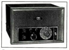
The dial on this crystal-synthesized International Crystal Mfg. Co., Executive shows an unmarked position between channels 22 and 23. In actuality, that tuned to non-channel 22A.
