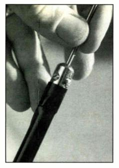
LENGTHEN the mobile CB whip to LOWER the best SWR readings.
