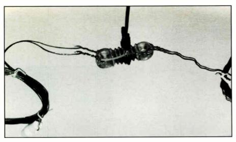
The center portion of a coiled-up dipole.
