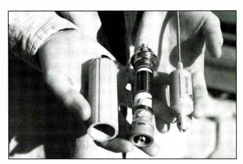
Here's a tapped base-load (left) and center-load on the right.
