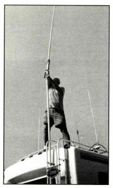
When a big base CB antenna gets water into it, you must remove it to drain out the water. WATCH FOR POWER LINES!
