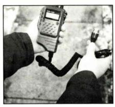
The RadioShack TRC-232 CB walkie-talkie comes complete with a handy vehicle power/antenna adapter. Simply remove the battery pack from the bottom of the radio, slide on the power adapter, plug in the cigarette lighter cord, connect your antenna, and you're on the air from your vehicle. In this configuration, the radio is only a bit larger than a standard mobile CB mic. The power cord isn't a flimsy cord either, and the plug is even fused.
