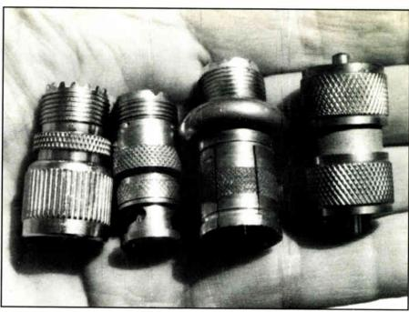
None of the coaxial cable plugs seen here are waterproof. They MUST be sealed.
