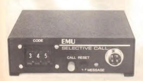
Emu Systems have developed a high-quality sel. call device which can transmit and receive on two different codes, giving greater flexibility when more than two units are used. The receive code is programmed internally and the transmit code selected by three switches on the front panel. The unit also features a message-received light, indicating a call has been received in the user's absence.
