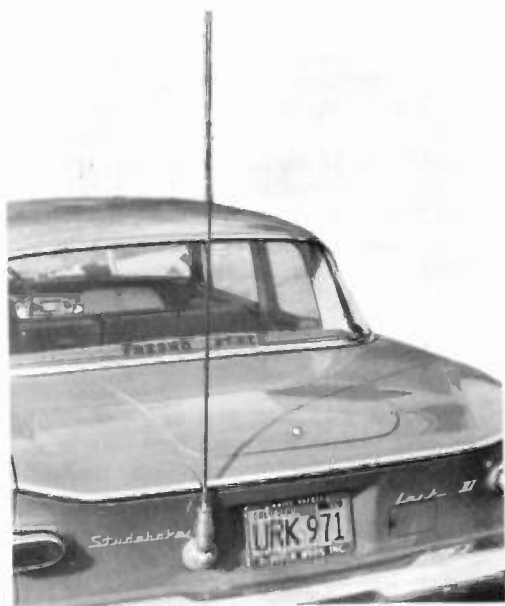
"49'er" whip mounted on Model "5" spring, Model "B" ball mount. This installation on 2817's mobile.
