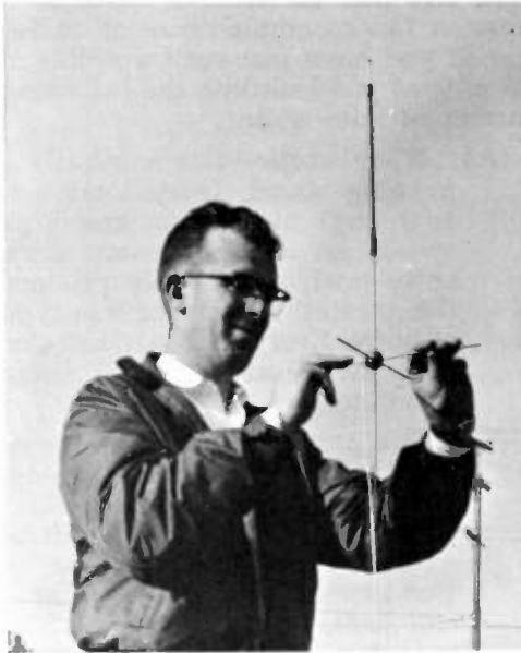
Engineer Lorry Henley positions the MP-1 on the Topper test whip. Unit resembles Sputnik with hub and four spokes!
