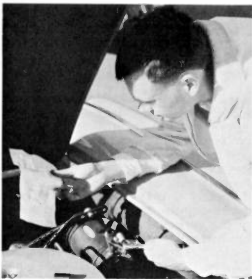
MOUNTING NOISE FILTER —with instructions provided by Ben Bortlett (see text), it's a mobile noise cinch as 12Q2339—unit 4 found out. The filter rests on the air cleaner, foreground.
