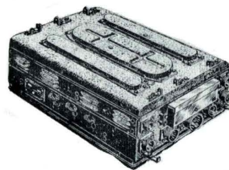
The BC-645 U.S. Army transceiver, the first mass produced set used on CB frequencies.
