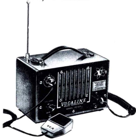
Vocaline's JRC400 Class B transceiver, the only Class B unit ever to gain any popularity whatsoever.
