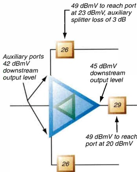
Figure 6: Input pads with downstream taps.
