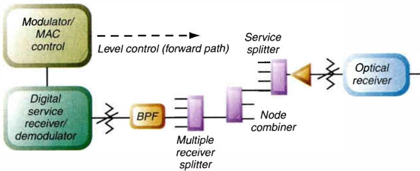
Figure 2: Closed-loop level control.
