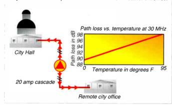
Figure 2: Reverse level adjustments are compensated for by AGC modules.
