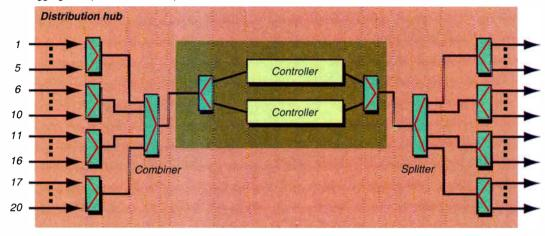
Figure 5: Example of cable node aggregation (RF concentration) for initial service introduction.
