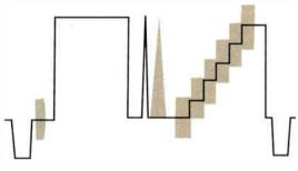
system, and the time it takes for the black-andwhite portion of the signal (luminance) to pass through a system. The amount of distortion is expressed in time in nanoseconds. If the number is positive, the chrominance is slower than the luminance. If the number is negative, the chrominance is faster.
