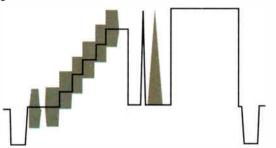
Figure 4: The NTC7 composite signal has some limitations for making color tests because its staircase exceeds 100 IRE and can cause a properly adjusted modulator to momentarily overmodulate.
