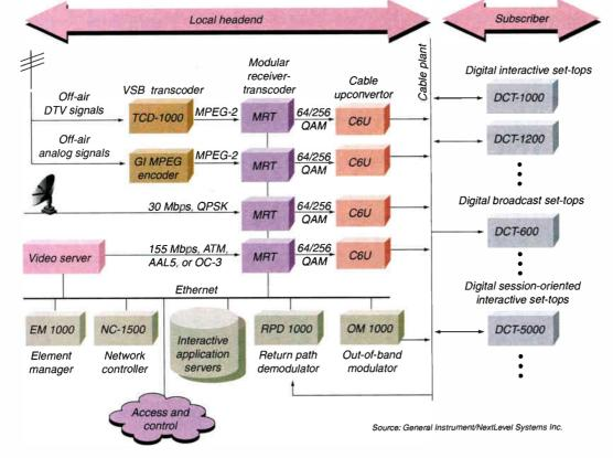
information to and from the subscriber. These RF channels are located in available channels in the forward spectrum, typically between 50 MHz and 550 MHz. In the reverse direction, RF channels bringing data back from the subscriber are generally situated in the 5 MHz to 30 MHz range. Newer and upgraded hybrid fiber/coax (HFC) cable systems are generally designed to extend the forward spectrum to 750 MHz and the reverse to 42 MHz.
