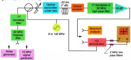
Figure 5: Notched noise plus CW carrier.
