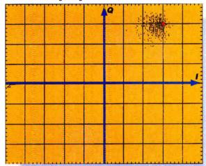
Figure 11: Signal state spreading of a 142 MHz carrier during noise load testing at high levels.
