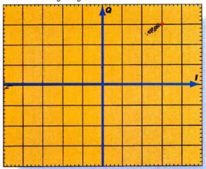
to the normal input level for these transmitters (+18 dBmV). For all three lasers, the effect of this out of channel signal is an almost identical, radial, compression of the wanted signal. An example measurement is shown in Figure 12.
