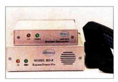
GADline's Subscriber Interface Unit 503-B brings voice/data communication into the home where it provides plain old telephone service (POTS). The larger unit features a battery backup.
