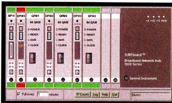
A mock-up of GI's new, rack-mounted SURFview data network management system.
