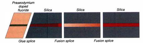
the results of their research. Using a single praseodymium doped fluoride fiber amplifier (PDFFA), they generated 16 dB of amplification in the optical domain and transmitted a 5 Gbps data stream at 1310 nm over 100 km of silica cable. While BT's experimental results demonstrated a technical solution, providing the telecommunications industry with a practical PDFFA required more creative research and engineering.
