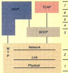
MTP = Message Transfer Part SCCP = Signaling Connection Control Part
