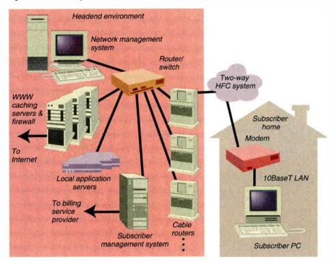
Figure 1: Network diagram for major components of broadband HFC data system
