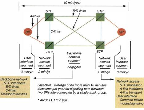
Figure 2: Reference model\* for Message Transfer Part (MTP) network downtime objective
