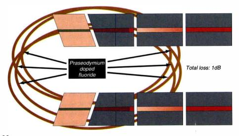
Having developed a suitable fluoride fiber, the next obstacle was developing a means to provide this fiber in a package compatible with silica fiber. This was not an easy task, considering that fluoride and silica fibers have such dissimilar characteristics. The key issues are illustrated in Figure 1. For amplification purposes, the fibers need to be spliced in a way that supports optical transmission in both the 1310 nm band and in the band of the pump frequency.
