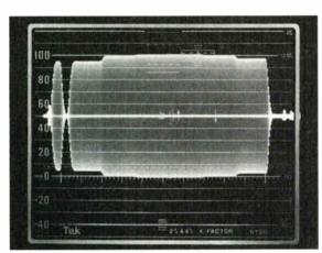
*Figure 2:* This modulated staircase signal exhibits a 10 percent differential gain error.
