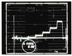
Figure 4: This is the waveform monitor single trace diff phase indicating 6 degrees of differential phase distortion.
