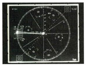
Figure 3: A vectorscope display showing a 5 degree differential phase distortion.
