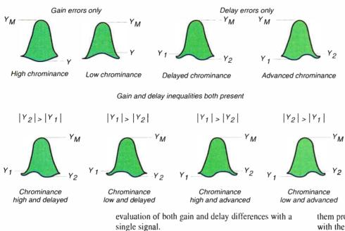
To check for chrominance-to-luminance gain and delay, use the waveform monitor's variable gain and
