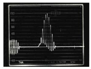
**Figure 5:** A sinusoidal distortion in the base of the 12.5T mod pulse indicates chrominance-to-luminance delay. In this example, chrominance is delayed by approximately 250 ns.
