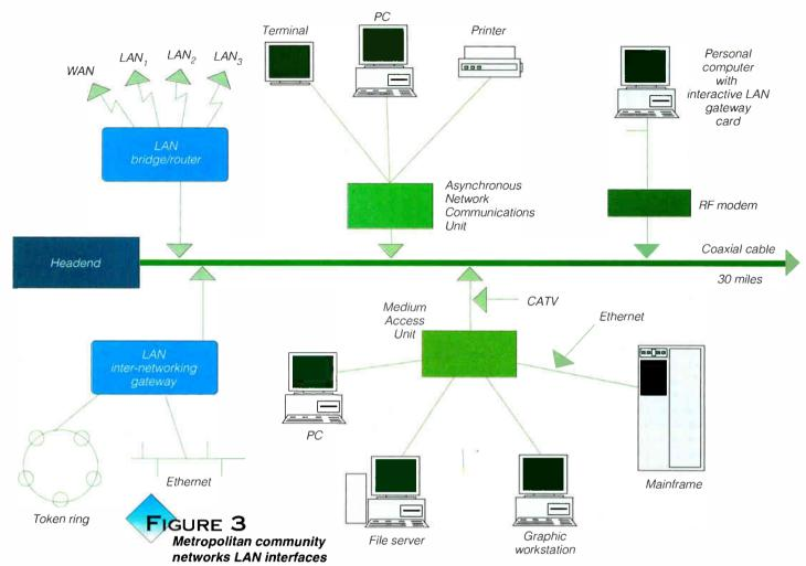
ranging from mainframes to IBM PC compatibles to Apple Macintoshes to Sun SPARCstations to terminals and printers, requires a variety of connectivity solutions from the perspective of a network provider. Physical medium interfaces are available for network connections to coaxial, twisted pair, fiber optic and even wireless.
