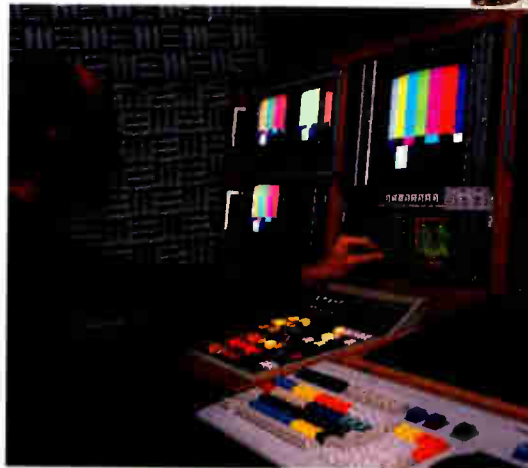
(ABOVE) THE CMP500 CABLE TELEVISION MEASUREMENT PACKAGE — COMPLETE BASEBAND VIDEO AND RF MEASUREMENT CAPABILITY, INCLUDING ALL FCC PROOF-OF-PERFORMANCE REQUIREMENTS.
