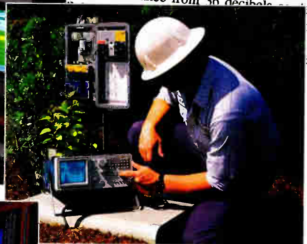
(ABOVE) THE 2714 CABLE TV SPECTRUM ANALYZER AUTOMATES ALL COMMON CABLE SYSTEM SPECTRAL MEASUREMENTS, INCLUDING THE FCC RF PROOF-OF-PERFORMANCE REQUIREMENTS.
