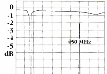
Low Off Notch Attenuation To At Least 450 MHz Type 3271ABH-8
