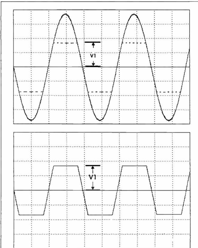
ILLUSTRATION OF  $I^2R$  LOSSES IN ZENER TYPE CLAMPING CIRCUIT
