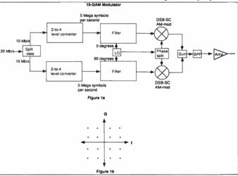
constraints over a given transmission path. The current HDTV proponents are convinced that HDTV will not be possible in less than about 20 Mb/ s total data rate. If we force this signal to be placed within a 6 MHz channel, we must use a modulation technique that will realistically provide a channel efficiency of 3.33 bits/ Hertz (20/6).
