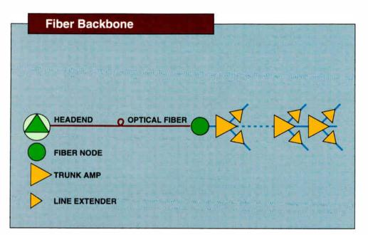
Conventional fiber backbone reduces active cascades as compared with coaxial trunk system. This improves picture quality and service reliability while extending system range. Sumitomo full bandwidth transmission and plug-in filters provide flexible split-channel loading. A/B switch provides system redundancy.
