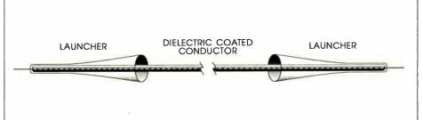
of a short rigid coaxial stub, the diameter of whose outer conductor is increased in a gradual taper to form a long, narrow funnel about one quarter wavelength in diameter at the mouth.
