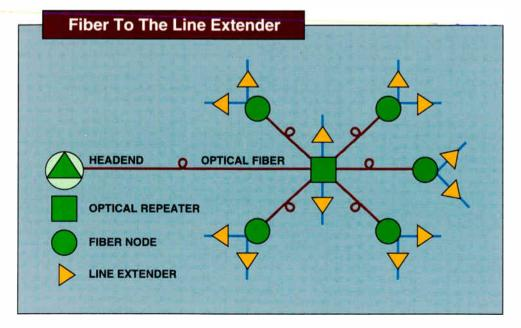
Sumitomo strand-mount optical repeater and secondary-node receiver eliminate need for trunk and distribution amplifiers. Resulting fiber-to-line-extender architecture minimizes active devices between headend and subscriber. Advanced design also minimizes maintenance, and allows expansion without backbone redesign or rework.
