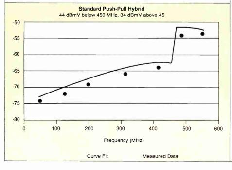
of the digital signals, they can be transmitted through the cable system at lower levels than the accompanying VSB/AM signals. This reduced loading results in improved amplifier performance for the AM channels. By taking advantage of this improved performance, it is possible to reduce the plant cost, compared to a traditional system with the same RF bandwidth carrying all VSB/AM channels.
