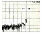
Brickwall HPF 6211HP-47/48 Passes Channel 80 Up, 50 dB Channel 47 Doun
