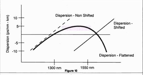
this minimum point is referred to as the zero dispersion wavelength and in many fibers is located at around 1300 nm. By employing special index profiles at the core/cladding interface it is possible to construct the fiber cable in such a way as to "shift" the zero (Figure 10).
