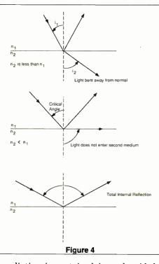
radiation is contained in and guided through the core. As mentioned earlier, there is a definite angle beyond which the optical energy will leave the core entirely. This is the critical angle. In other words, if the light enters the core at angles greater than the critical angle, the light rays will escape into the cladding and not be transmitted through the core.
