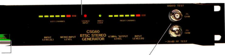
RF output purity, stability and video quality can be monitored with front panel video and RF output test ports.
