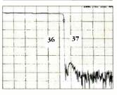
Brickwall LPF 6211LP-36/37 Passes Channel 36 Down, 50 dB Channel 37 Up
