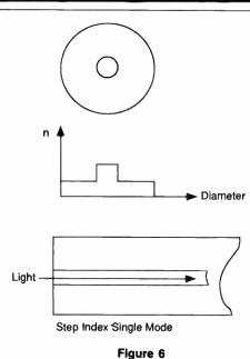
fined, an acceptance cone can be formed in which light entering within this cone will be transmitted while light entering at steeper angles will not. An increase in the NA results in an increase in the optical energy that can be accepted into the core. However, a large NA leads to more paths of light resulting in an increase in dispersion (to be discussed later). The NA for step index fiber is a function of the two
