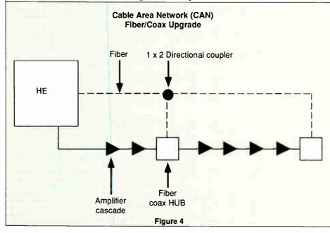
It uses fiber to carry video signals from the headend site to various nodes located within an existing coaxial distribution system. By bypassing long coax segments, this application eliminates the need for extended amplifier cascades. The in-place amplifiers are redirected and used to extend a higher quality signal further into the system with no additional expenditures for active equipment.
